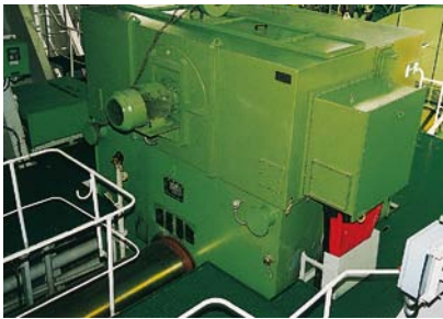
Shaft alternator 4500 kW, 65 - 94 rpm
