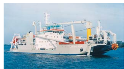
Cutter dredger "Batang Anai"
