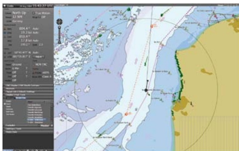
NACOS Platinum: ECDIS display with Radar overlay
