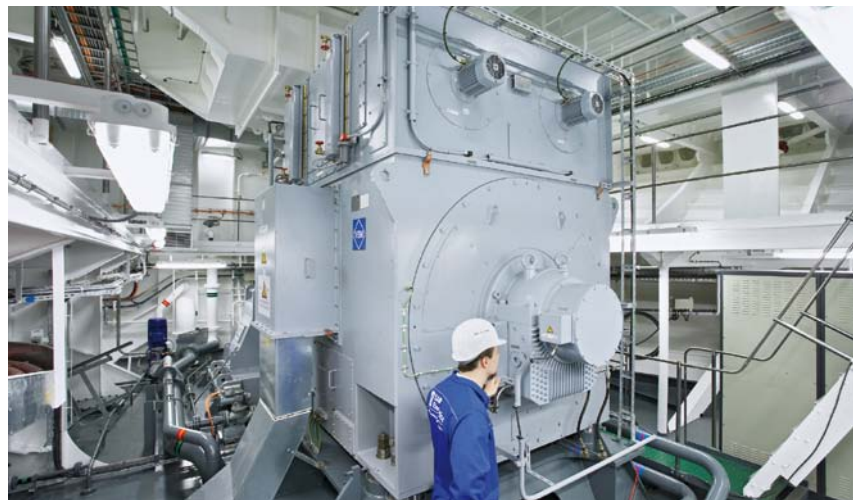
Propulsor motor 11 MW, 720 rpm on double ended ferries for BC Ferries
