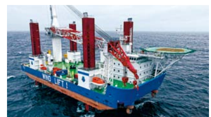
Jack-up vessel "Windlift 1"
