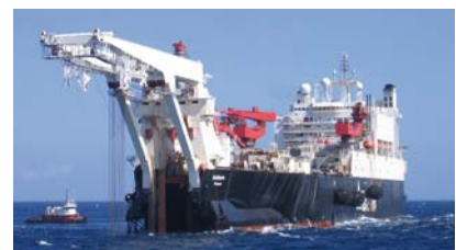
Pipelaying vessel "Solitaire"
