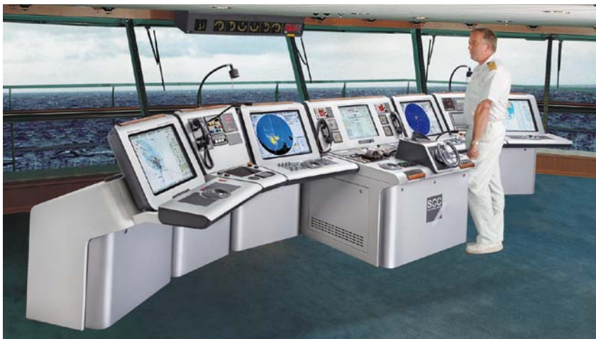
Ship Control Center (SCC) - bridge concept with high level integration
